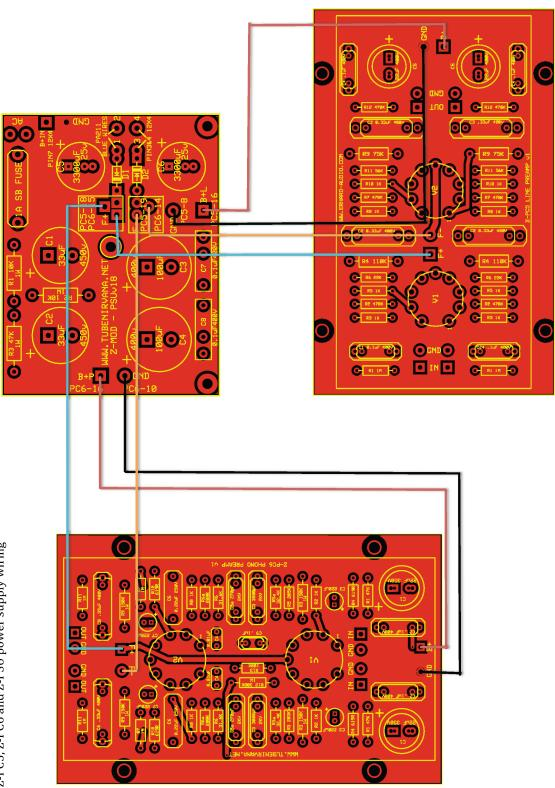
Z-PC5, Z-PC6 and Z-PSU power supply wiring
