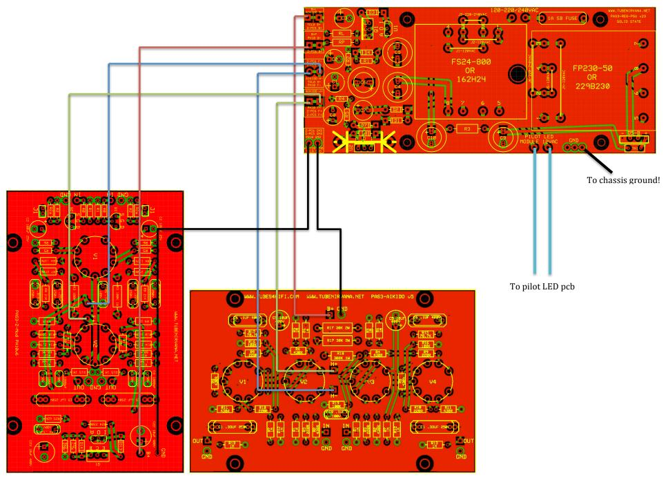
Power supply connection diagram for Solid State Regulated Power Supply v23 with Z-Mod PH10 and AIKIDO.
