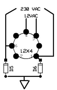
add D5 and D6 to pins 1 and 6 on 12X4 rectifier to ground as shown
