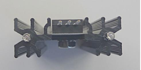
Note one side of the heatsink has narrowed fins, install the LM350 on THAT SIDE!
