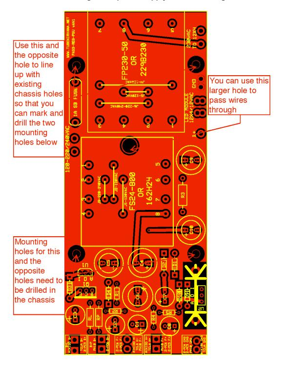
As an alternative to drilling holes in your chassis, you can use the optional self adhesive pvc printed circuit board standoffs included in the kit!..
